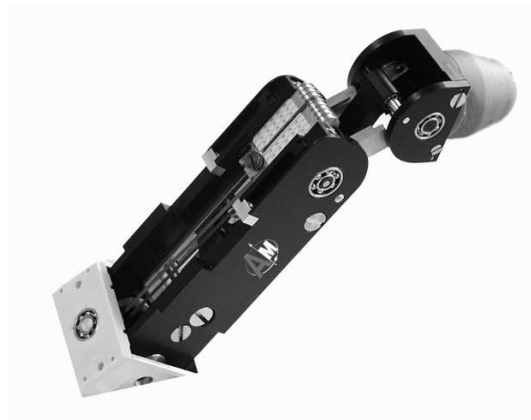
Fig. 1. Artificial finger actuated by SMA wires. Courtesy of H. Ulbrich.
